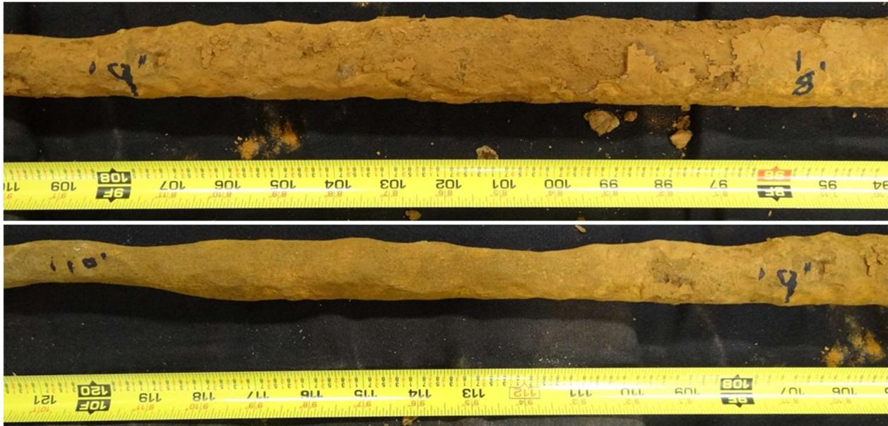
**Figure 9: Different corrosion rates along an anchor shaft due to vertical variations in soil corrosivity**
