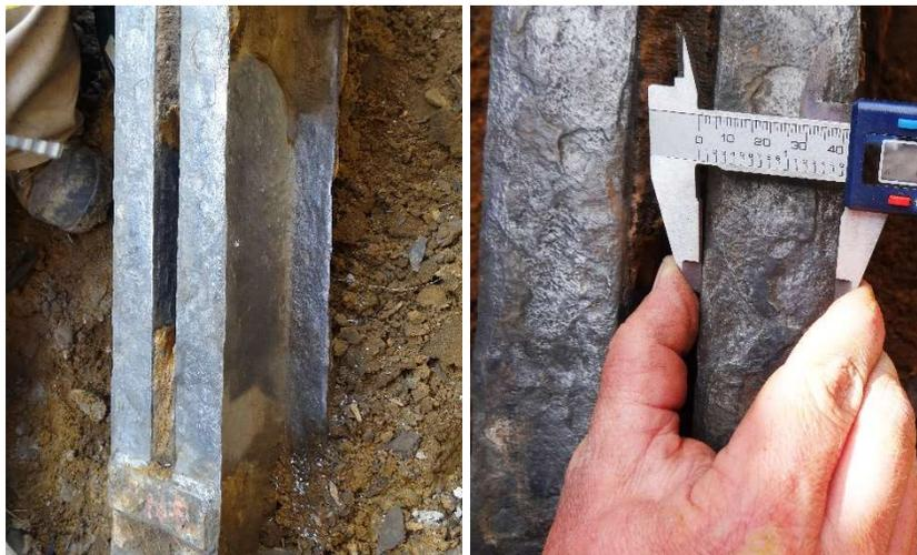
**Figure 6: Excessive material loss on an anchor shaft due to stray current corrosion**
